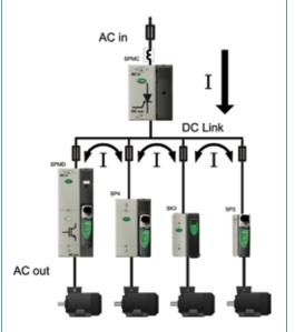
Drives from the Unidrive and Commander families can be connected on a common DC bus system, in order to circulate energy between drives with opposing energy flow, supplied from a controlled rectifier input (SPMC), an active input (SPMA or SPMD) or an existing DC source.
